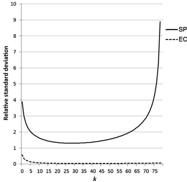
**Fig. 2.** For  $N = 80$  and varying  $k$ , the solid curve shows the relative standard deviation of  $s_k^{SP}$ . The dashed curve shows the upper bound from Eq. (4) of the relative standard deviation of  $s_k^{EC}$ .
